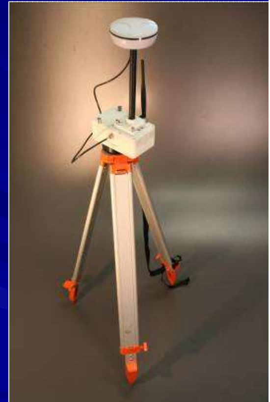
RTK Base station PCM, tripod, and radio telemetry
